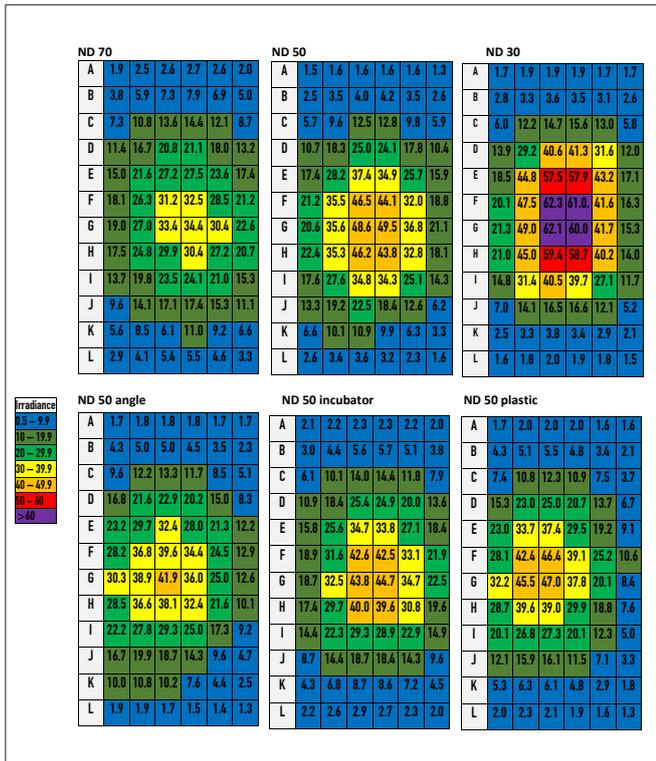
Fig. 5. The irradiance map of the Ningbo David phototherapy light in different settings. (ND 70 = Ningbo David at 70 cm; ND 50 = Ningbo David at 50 cm; ND 30 = Ningbo David at 30 cm; ND 50 angle = Ningbo David at 50 cm at an angle; ND 50 incubator = Ningbo David at 50 cm through an incubator; ND 50 plastic = Ningbo David at 50 cm through food-grade plastic.)
