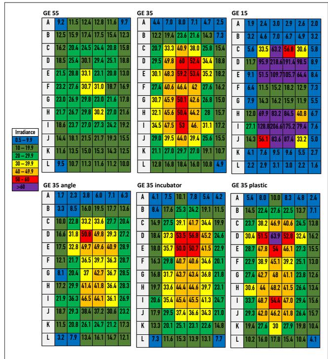
Fig. 4. The irradiance map of the General Electric phototherapy light in different settings. (GE 70 = General Electric at 70 cm; GE 50 = General Electric at 50 cm; GE 30 = General Electric at 30 cm; GE 50 angle = General Electric at 50 cm at an angle; GE 50 incubator = General Electric at 50 cm through an incubator; GE 50 plastic = General Electric at 50 cm through food-grade plastic.)
