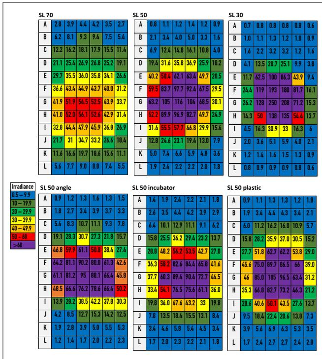
Fig. 3. The irradiance map of the Servolite phototherapy light in different settings. (SL 70 = Servolite at 70 cm; SL 50 = Servolite at 50 cm; SL 30 = Servolite at 30 cm; SL 50 angle = Servolite at 50 cm at an angle; SL 50 incubator = Servolite at 50 cm through an incubator; SL 50 plastic = Servolite at 50 cm through food-grade plastic.)
